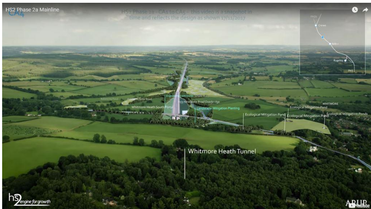
Figure 7.4d View over Whitmore Heath to tunnel south portal approach and A53 overbridge; Common Lane and Snape Hall Road south widened to 5 metres.
