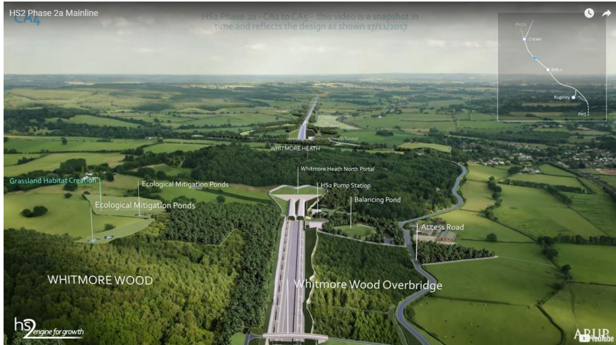
Figure 7.4d View over Whitmore Heath to tunnel south portal approach and A53 overbridge; Common Lane and Snape Hall Road south widened to 5 metres.
