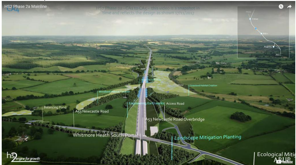
Figure 7.4e A53 overbridge, Whitmore south cutting and approach to Whitmore Heath tunnel south portal.
