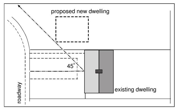
SD9. New buildings that are to be sited facing the principal windows of existing properties should be designed so that there is no obstruction to daylight beyond a vertical angle of 45° measured from the mid point of the nearest window(s)) of any adjacent property.
